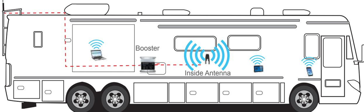
The Booster captures the signal from outside vehicle and boosts it to the phone.
