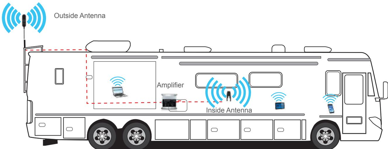
The Amplifier captures the signal from outside vehicle and boosts it to the phone.
